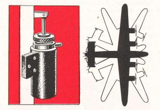
This is accomplished by loosening the locknut on the dashpot, turning the knurled ring up or down until hunting ceases, then tightening the locknut.
