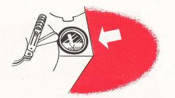
4. Have the bombardier disengage the autopilot clutch, center PDI and lock it in place by depressing the directional control lock. The PDI is held centered until the pilot has completed the engaging procedure. Then the autopilot clutch is re-engaged, and the directional arm lock released.
