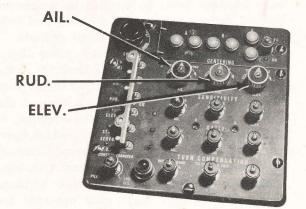
5. Engage the autopilot. Put out aileron telltale lights with the aileron centering knob, then throw on the aileron engaging switch. Repeat the operation for rudder, then for elevator.
