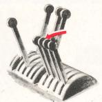
7. Mixture Auto-rich. Copilot puts mixture control in "AUTO-RICH," booster pump off.
