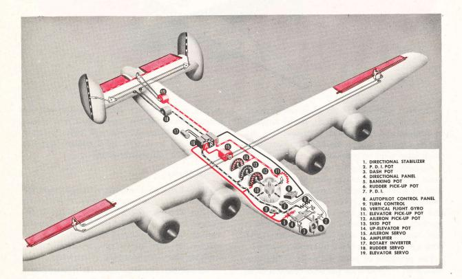
aileron, rudder, and elevator Servo units cause each of these units to operate its respective control surface just enough to bank and turn the airplane back to a level-flight attitude.
