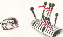
4. Application of Power. Copilot adjusts mixture controls on other engines and increases rpm. Pilot increases manifold pressure. Actions of pilot and copilot are approximately simultaneous, but the increase of mixtures and rpm should always precede the increase in manifold pressure.
