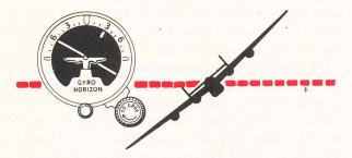
should bank  $30^{\circ}$ , as indicated by artificial horizon. If it doesn't, remove cap from aileron trimmer and adjust trimmer until a  $30^{\circ}$  bank is attained. Then, if turn is not coordinated (inclinometer ball not centered), adjust rudder trimmer to center ball. Make final adjustments with both trimmers and replace caps. Set turn control at zero to resume straight and level flight; then re-center.
