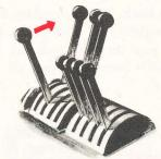
4. Throttle Cracked. Pilot cracks throttle.
