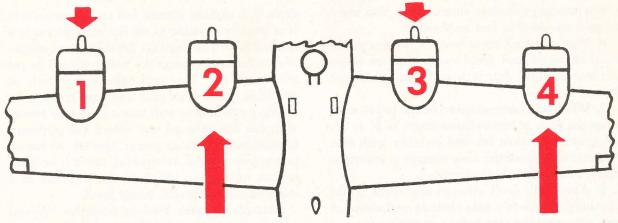
No. 2 Dead—You lose generator, heaters (for pilot, copilot and top turret gunner) and vacuum pump. Switch vacuum to No. 1.
