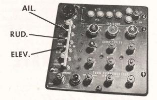
6. Make final autopilot trim corrections. If necessary, use centering knobs to level wings and center PDI.
